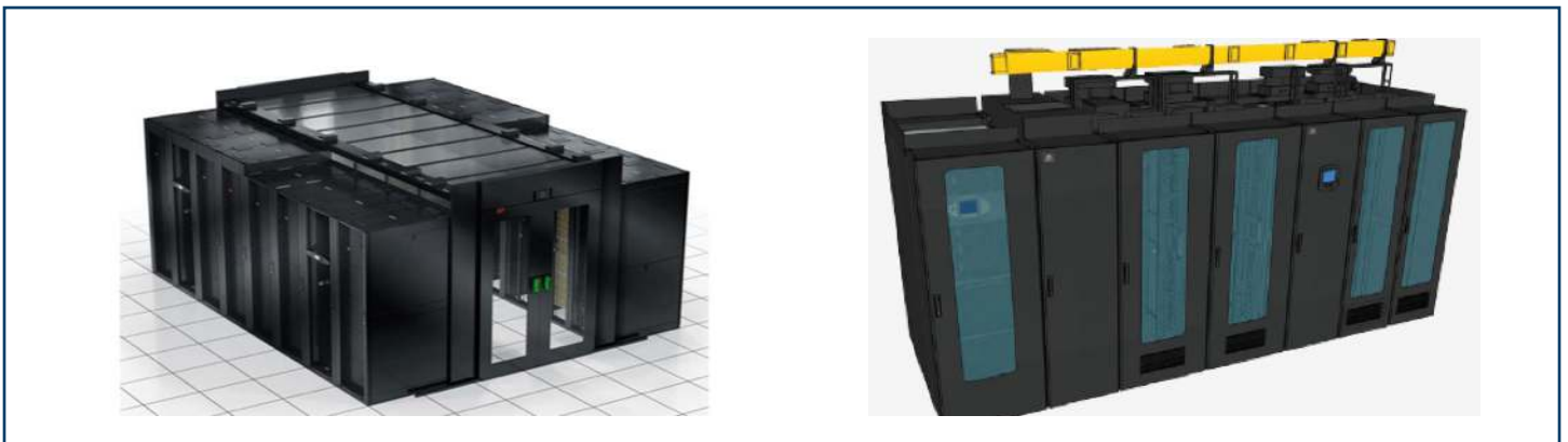
Figure 4. Examples of indoor rack line-ups or pods to suit the in-building deployments. Pictures are of APC Schneider Electric's EcoAisle™ product line (left). This lineup is built up from a series of single rack or cabinet products with the appropriate aisle containment infrastructure, power distribution, and possibly in-row coolers. Another indoor deployment approach is Vertiv's SmartRow™ system (right). This system is smaller in size and is built from a series of self-contained cabinets with in-row coolers, power, and fiber distribution.*
